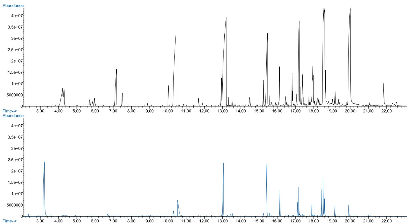
**Figure 8.** Total Ion Chromatograms. Top: (TICs) of 5 mL whisky brand A (23% v/v, 1:1 diluted with HPLC water) extracted with EG-Silicone Twister split 1:20; bottom: 20 µL of whisky brand A (46 % v/v); direct injection (LVI), splitless.
