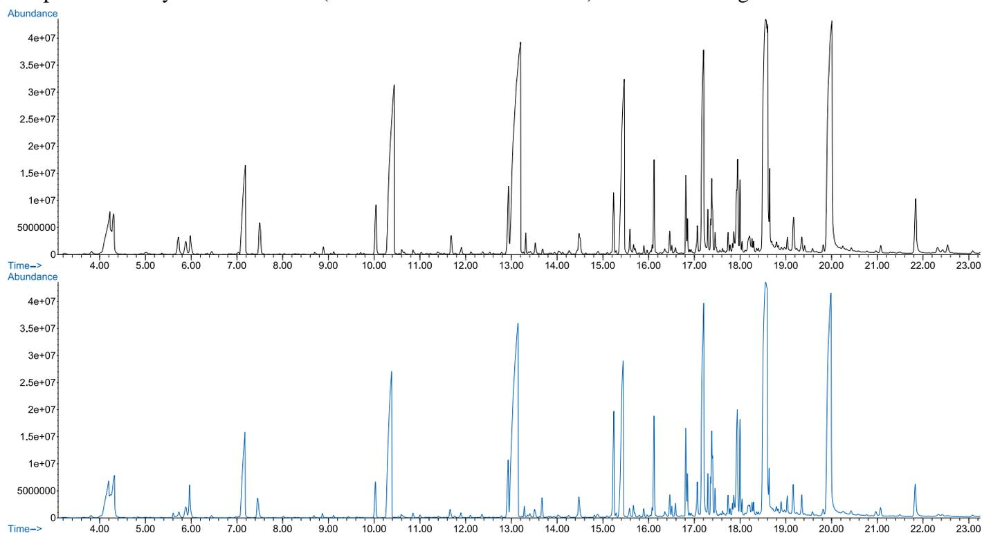
**Figure 5.** Total ion chromatograms of 5 mL samples of two whisky brands (1:1 diluted with HPLC water) extracted with SBSE using EG-Silicone Twister. Top: Brand A (23 % EtOH v/v), bottom: Brand B (20 % EtOH v/v).
