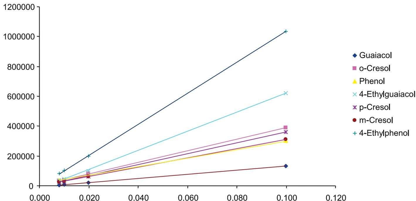
**Figure 7.** Calibration curves for seven phenolic compounds obtained with EG-Silicone Twister at 8, 20, 40, and 100 ng/mL in 20 % (v/v) ethanol/water matrix.
