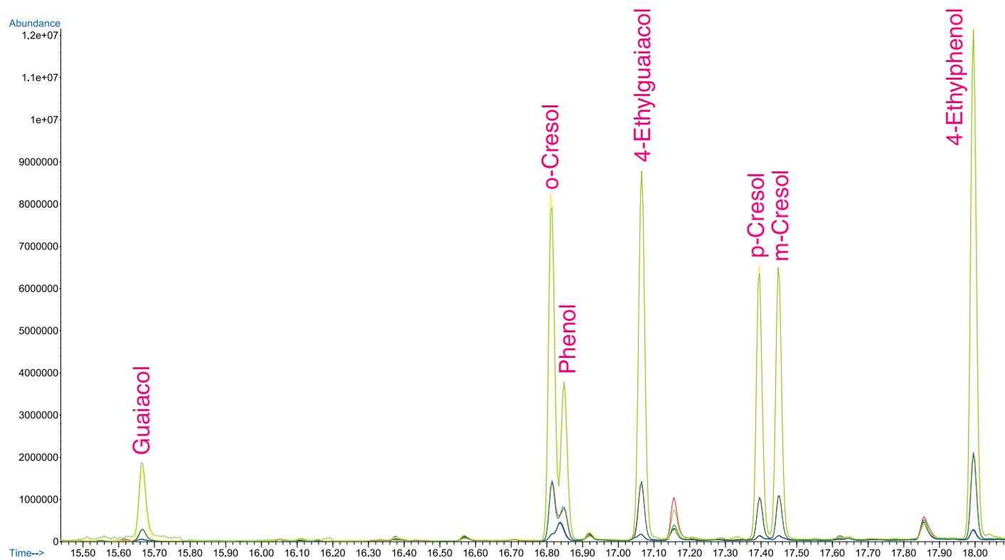
**Figure 4.** Total Ion Chromatograms (TICs) obtained with SBSE using EG-Silicone Twisters showing seven phenolic compounds at 0.01, 0.1 and 1.0 ng/ $\mu$ L respectively in 5 mL synthetic whisky [20 % (v/v) ethanol/water, pH = 3], split 1:20.
