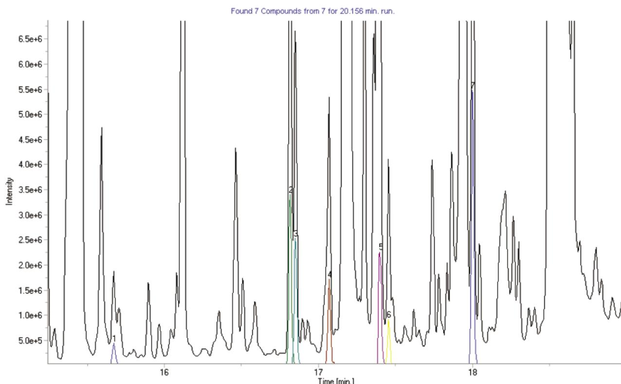
**Figure 6.** Overlay chromatograms of RIC and TIC of a 5 mL sample of whisky brand A (1:1 diluted with HPLC water, 23 % EtOH v/v) obtained with SBSE using the EG-Silicone Twister.
