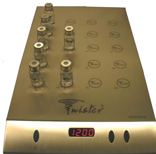
Figure 3. Dilute 1 mL acetonitrile extract with 0.1 M \text{NaHCO}_3 and perform SBSE.
