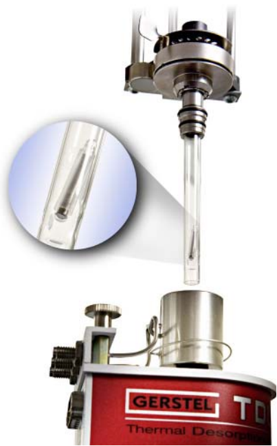
Figure 4. Desorb GERSTEL Twister using Thermal Desorption Unit.
